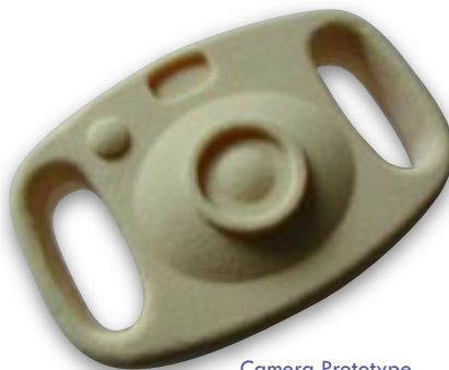
Camera Prototype (High Density Foam)
